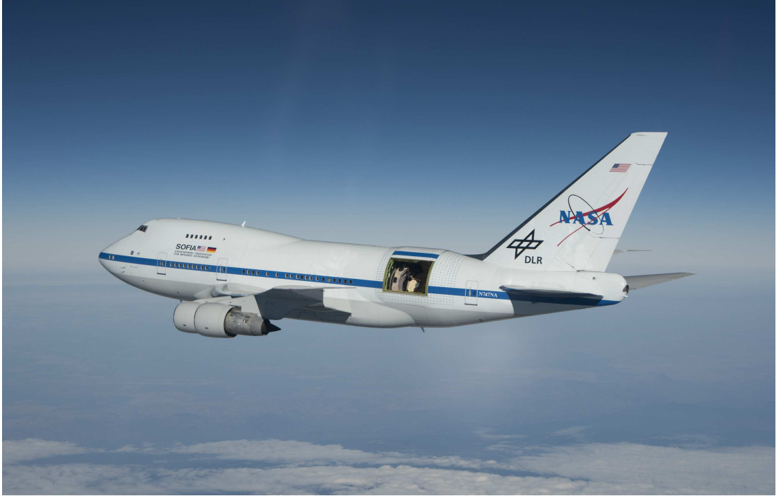
Figure 3.2: NASA’s Stratospheric Observatory for Infrared Astronomy 747SP aircraft flies over Southern California’s high desert with the large door of its 2.5 m German-built telescope open. Image Credit: NASA/Jim Ross
